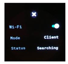
The aim here is to have the your smartphone and the Waylens Horizon connected to the same network. To do so, we're going to tap on "Mode" and switch to the Client option, which basically allows the camera to pick up any surrounding Wi-Fi signals.
